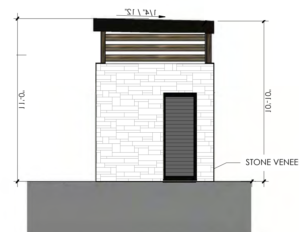
5 TYP. DUMPSTER SIDE ELEVATION 1/4" = 1'-0"
