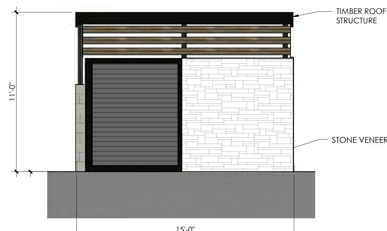
4 TYP. DUMPSTER ENCLOSURE ELEVATION 1/4" = 1'-0"
