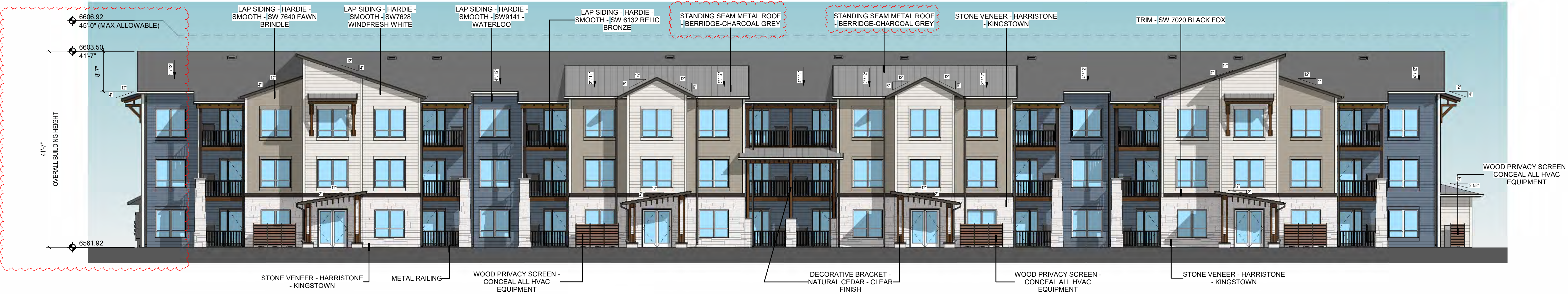
1 BUILDING TYPE 6 - FRONT ELEVATION (COLOR) MDP 3/32" = 1'-0"
