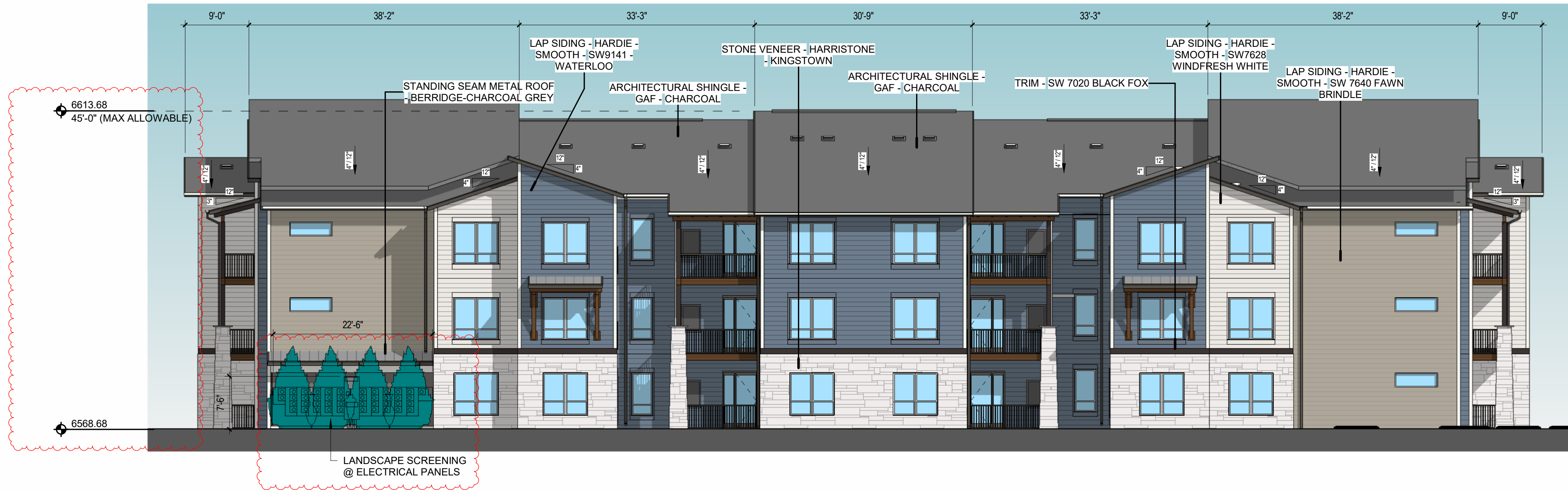
2 BUILDING #7 - BACK ELEVATION - COLOR MDP 3/32" = 1'-0"
